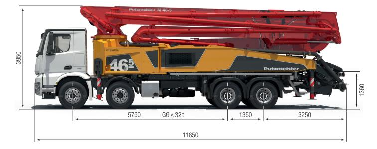
Note: Standard version. Dimensions and weights depend on truck, pump model and equipment. Dimensions in mm, MB-Arocs 4143 as example. For illustration only.
